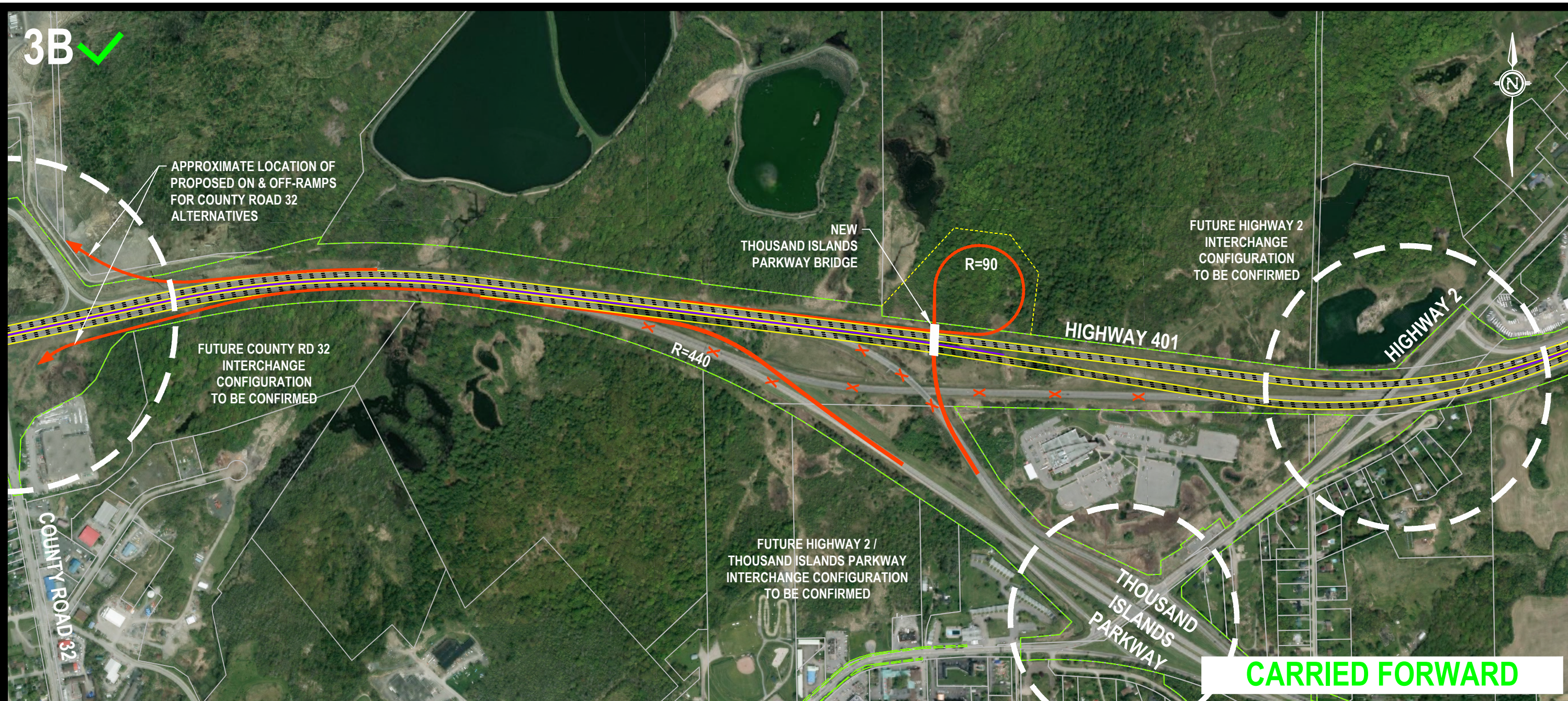
ALTERNATIVE 3B - WESTBOUND LOOP ON-RAMP AND REALIGN HIGHWAY 401 EASTBOUND LANES
